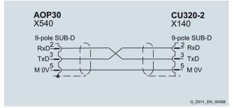
Assignment of the serial plug-in cable
